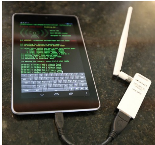
Figure 31: Pwn Pad – a commercial grade penetration tablet 11
