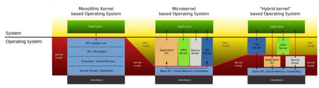
Figure 2: Monolithic & Microkernel structures
