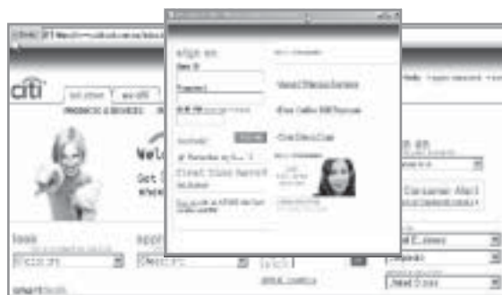
Figure 1: Spoofed pop-up with phony login visually on top of a real site.
